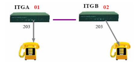
(Assume both ITGs have a FXS port on port #3 with a phone set connected.)
